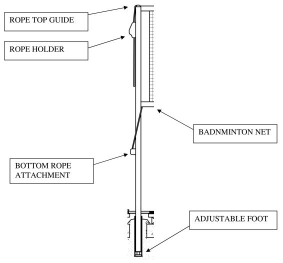
The net rope goes through the top guide and down to the holder to keep in place. The bottom rope attachment is tied off. The adjustable foot is to allow adjustment in case the sleeve depth is slightly off to allow net height to be adjusted to 5' 1".
