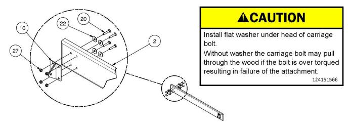
2. Install the chain support brackets onto the top wood pad using the hardware shown in the above illustration.
