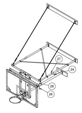
The final step of the assembly is to level the frame extension arm by adjusting the chain tension with the turnbuckles. It is important to not over adjust the chains as this causes undue stress on the chain anchor points. Chain tension should be no more than enough to level the side frame tubes.
