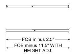
Slide the extension tube until the distance from the wall to the face of the board bracket is equal to the FOB minus 2.5" or FOB minus 11.5" when a height adjuster is to be used. Install the set screw (Item 29) into the outer extension tube and lightly tighten the set screw.
