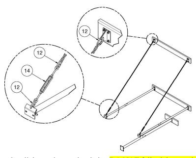
Install the 5O chains on each side of the unit. Attach the chain to the upper chain supports with the 5/16" quick links. Make sure the links are fully closed and tightened.
