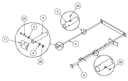
Slide the top inner extension pipes into the top outer extension pipes.
