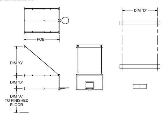
**Note:** The upper wood pad with the chain anchors should be mounted in the same plane as the two frame mounting wood pads. The load information for the upper chain anchor is based on the wood pad located in the same plane. Contact the manufacturer for correct reaction loads if there is a wall condition that does not allow the wood pads for the chain anchors to be in the same plane as the frame pads.
