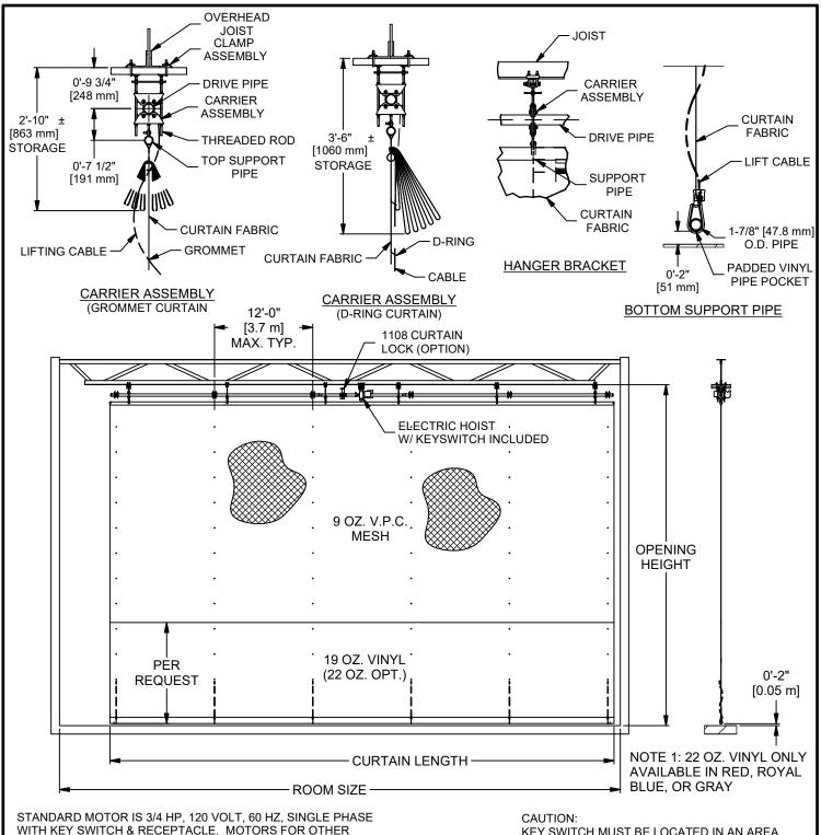
STANDARD MOTOR IS 3/4 HP, 120 VOLT, 60 HZ, SINGLE PHASE WITH KEY SWITCH & RECEPTACLE. MOTORS FOR OTHER POWER REQUIREMENTS ARE AVAILABLE. SEE SPECIFIC MOTOR SPECIFICATION DRAWINGS.
