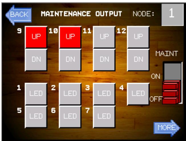
Here it shows that relays 9 UP and 10 UP are energized (due to their status as a toggle, specific to each system).
