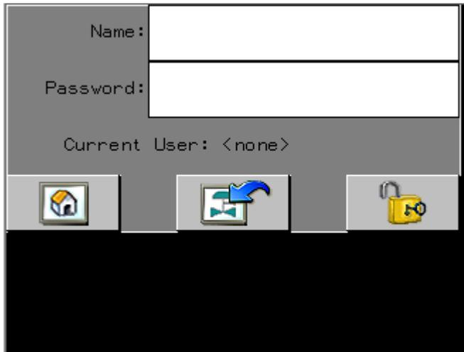
From here tap in the Name: field and enter ADMIN using the on-screen keypad.
