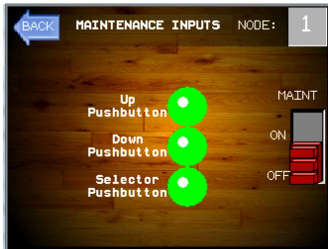
Pressing MORE a second time will take the operator to the INPUT page where diagnostics can be performed on the manual tethered switch. To diagnose, the
