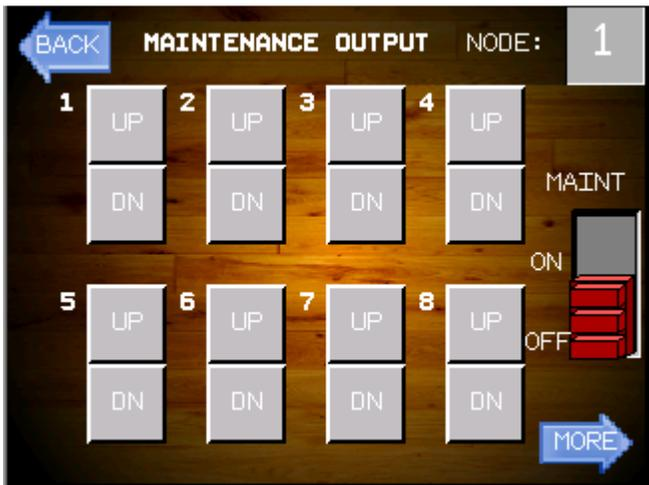
The components on this screen are used for troubleshooting and isolating outputs for testing purposes.
