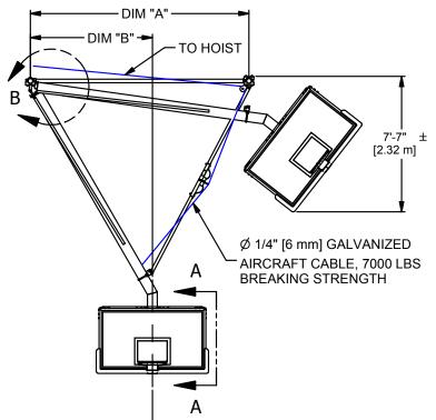
Dimensions "A" & "D" are shown for maximum elevation of the truss range and may vary to fit the exact attachment elevation and building structure.
