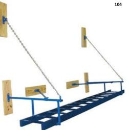
MODEL 104 HORIZONTAL LADDER is constructed of 1 5/8" diameter heavy wall tubing • Support frame is fastened to 2" x 6" wood boards sealed and varnished that are mounted to the wall • Ladder rungs are 1" diameter steel tubing • Includes grey powdercoat finish.
