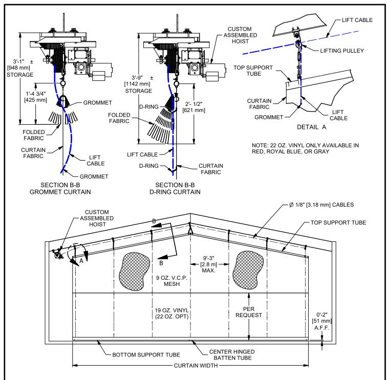
STANDARD MOTOR IS 3/4 HP, 115 VOLT, 60 HZ, SINGLE PHASE WITH KEY SWITCH & RECEPTACLE. MOTORS FOR OTHER POWER REQUIREMENTS ARE AVAILABLE. SEE SPECIFIC MOTOR SPECIFICATION DRAWINGS.
