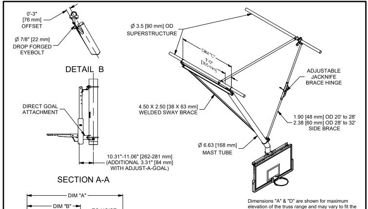
TO HOIST [2.32 m] Ø 1/4" [6 mm] GALVANIZED AIRCRAFT CABLE, 7000 LBS **BREAKING STRENGTH** - DIM "D" –
