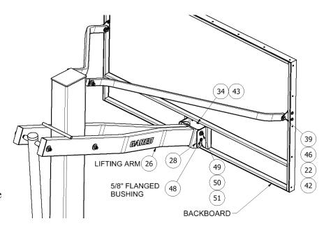
3. Continue holding board in a vertical position and install the ½ x 8" Bolt, #48, Flat Washer and Lock Nut as shown.
