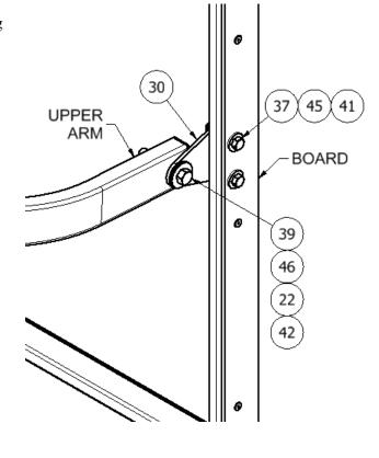
4. Snug all 7/16" Bolts to remove clearance. **Do not torque**.
